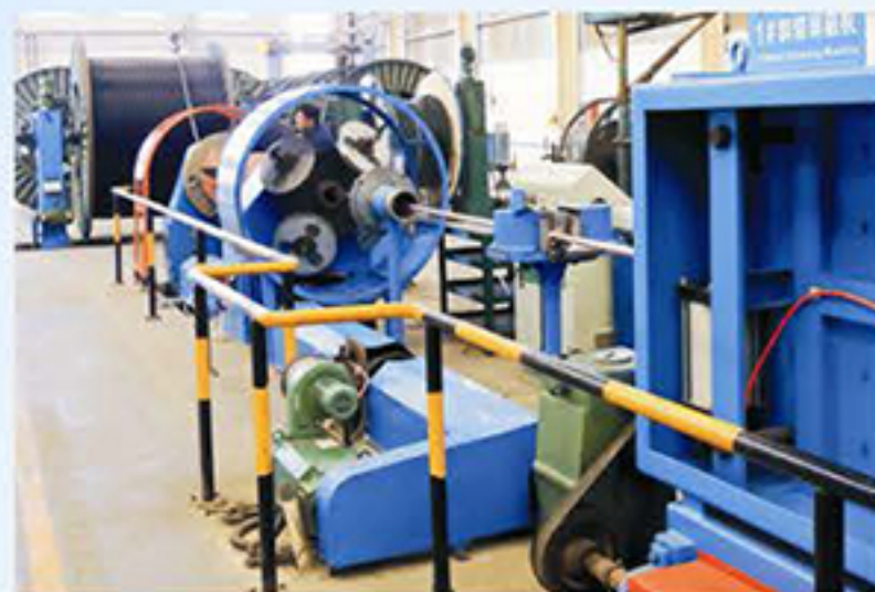
Copper tape screen machine
