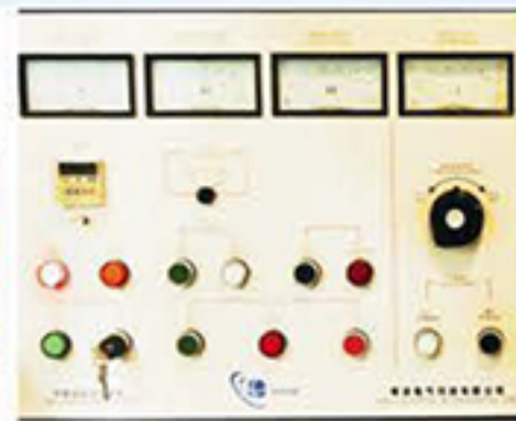
AC Voltage testing system
