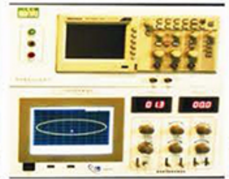
Partial Discharge Test System for MV cable
